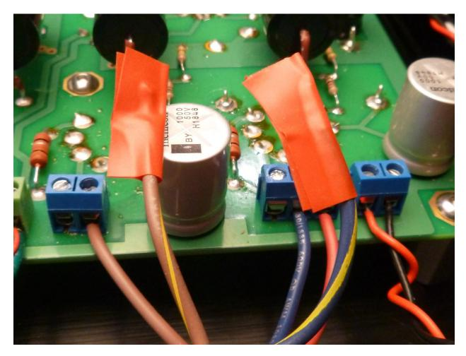
Loosen the connector block screws for the **brown-yellow** & **blue yellow** output transformer wires, **both channels**. Tape over the ends but give them a wide berth when the amp is running. There will still be about **300 Volts DC** on them! In fact, two layers of tape would be advisable.
