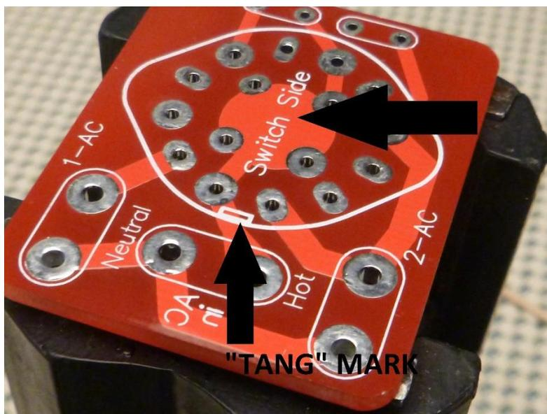
Assemble the switch to the board with the locating "TANG" on the switch positioned as shown.
