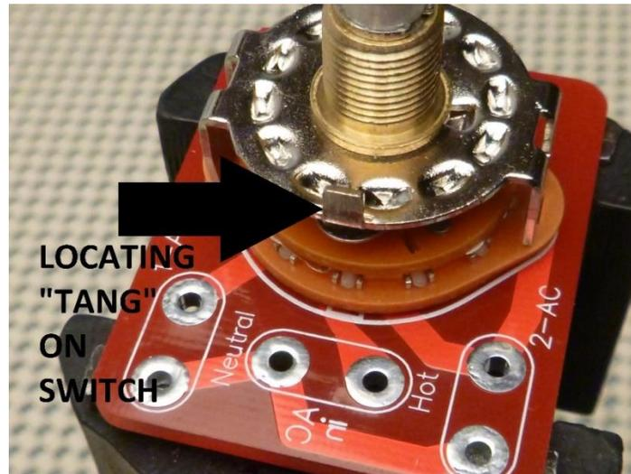
Solder the switch to the board. All of the holes on the Tubecad boards are plated through. Meaning, that if there are traces or pads on both sides (there usually is) there is copper connecting them through the holes. But very occasionally the plating through will be missed.
